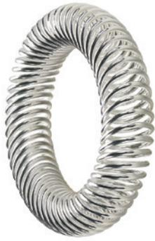
The Bal Spring® canted coil spring is a versatile component that mechanically fastens, conducts electricity, and shields sensitive electronics from the harmful effects of electromagnetic interference (EMI), and radio-frequency interference (RFI). The spring's independent coils, which serve as multiple contact points for optimal current carrying capability in electrical and shielding applications, ensure consistent, reliable connection—even under shock and vibration.
